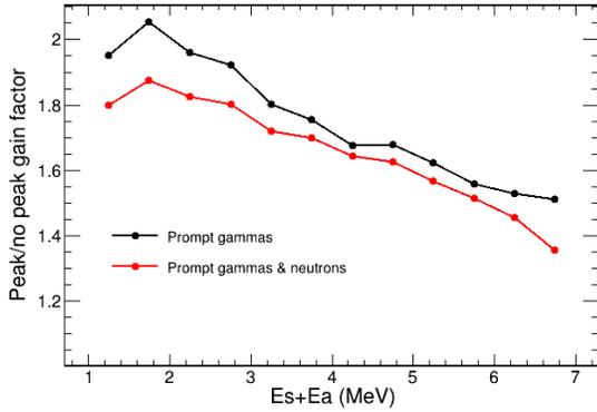
Fig. 1. Gain factor ratio as a function of the add-back deposited energy. The black and red lines represent, respectively, the results with only  $\gamma$ -ray events and including neutron events.
