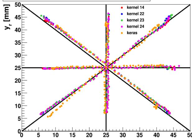
Position reconstructed Diagram for 15 mm  $\text{LaCl}_3$  crystal [Cov-svr(L)]
