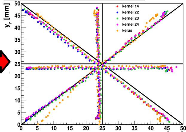
Position reconstructed Diagram for 25 mm  $\text{LaCl}_3$  crystal [Cov]
