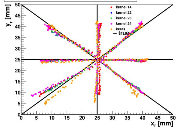
Position reconstructed Diagram for 20 mm  $\text{LaCl}_3$  crystal [Cov]
