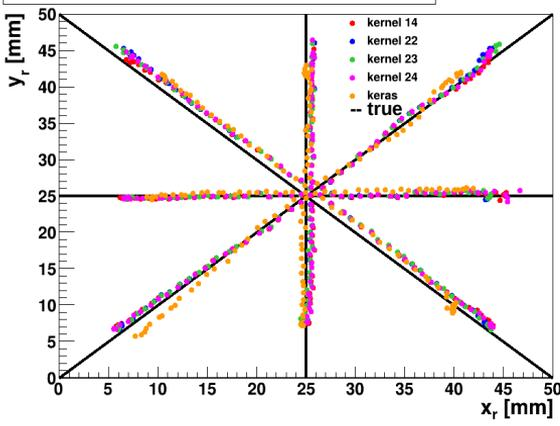
Position reconstructed Diagram for 30 mm  $\text{LaCl}_3$  crystal [Cov]
