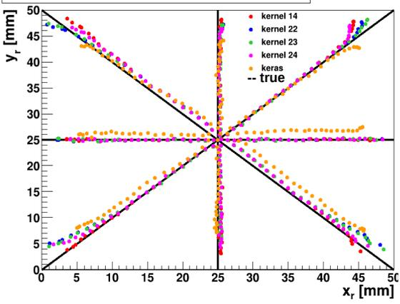
Position reconstructed Diagram for 15 mm  $\text{LaCl}_3$  crystal [Cov]
