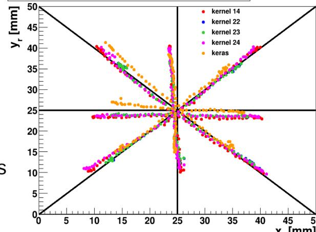
Position reconstructed Diagram for 25 mm  $\text{LaCl}_3$  crystal [Cov-svr(L)]
