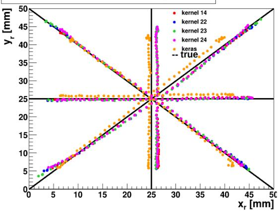
Position reconstructed Diagram for 25 mm  $\text{LaCl}_3$  crystal [Cov]
