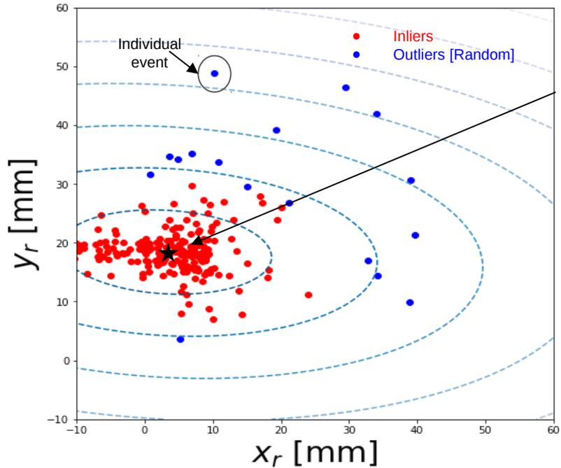
Reconstructed positions from the different models in the individual irradiations were fitted using the **robust covariance method** [1].
