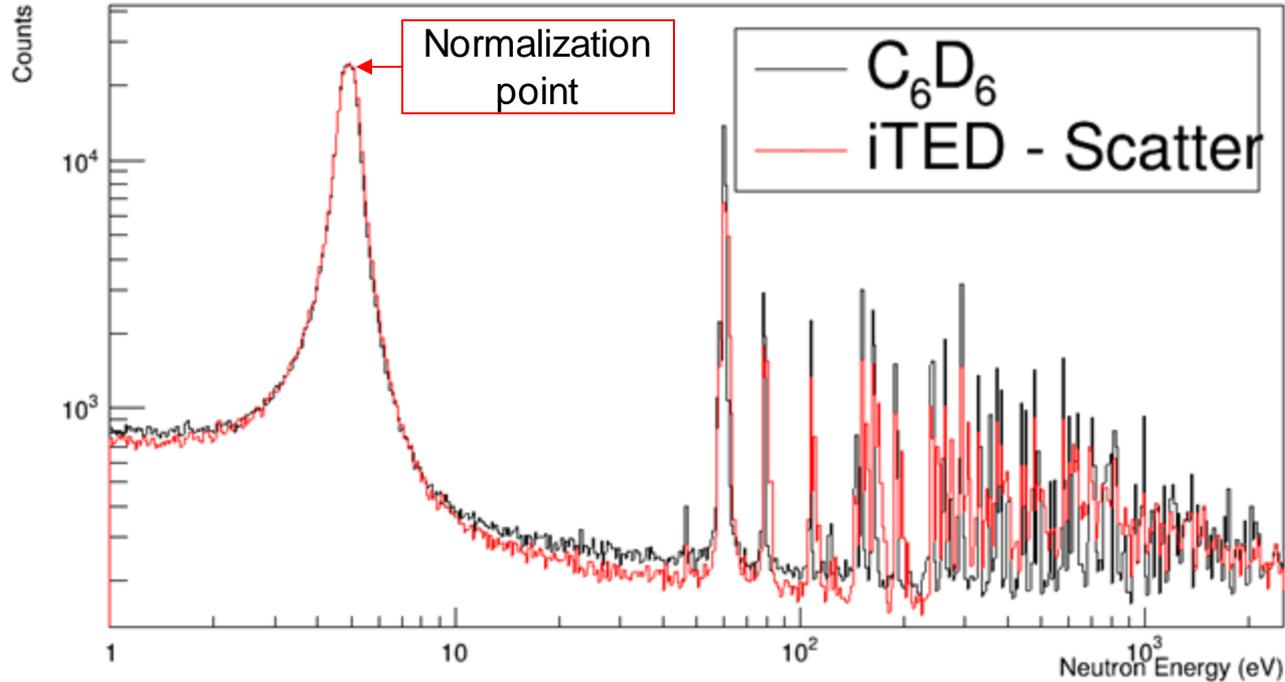
At first sight both TOF spectra look similar, however if we look in more detail in the high neutron-energy range a splitting and broadening of the narrow resonances can be observed in the i-TED data (next slide)
