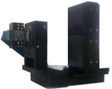
2018 i-TED prototype tested (3 LaCl 3 crystals, 192 channels)
