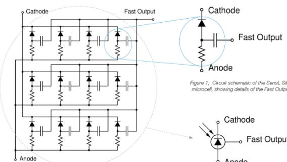
Figure 1. Circuit schematic of the sensL SPM microcell, showing details of the Fast Output.
